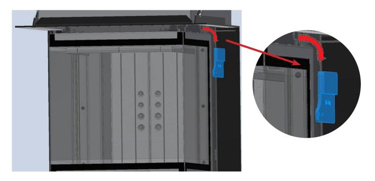
3. On the other side, also remove the M5 screws (using a 3mm allen key) that secure the door weight in place
